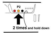
1- Press the push button **P2 two times and hold** it down, the buzzer will make a beep each time and then sound continuously.
