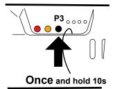
Push the push-button **P3 once and hold** it down for 10 seconds. The light turns on with a warm white colour and after 10 sec. it will flash once. The light will turn off at the release of the push button.
