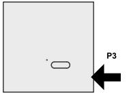
1- Press the button P3 located inside the already memorized transmitter. The enabled receiver sound continuously.
