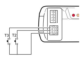
The Master receiver has two manual push buttons for wired command with the following functions:
