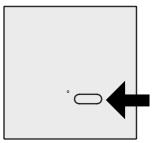
2- During the sound press the pushbutton which has to be memorised; the memorization is indicated by the intermittently sound of the buzzer. Function available for all type of transmitters
