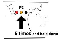
1- Press the push button **P2 five times and hold** it down, the buzzer will make a beep each time and then sound continuously.
