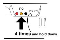
1- Press the push button **P2 four times and hold** it down, the buzzer will make a beep each time and then sound continuously.
