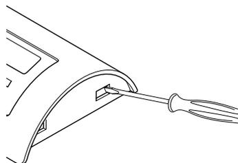
Press on the side tabs to open the bottom case
