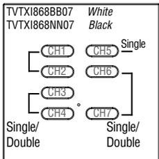
**Single / Double button commands (ON, OFF, ON/OFF/Dim, Open/Stop/Close, ...)**
