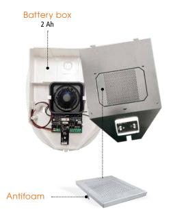
**SR Series** sirens are available in 2 different versions: SR136 and SR136 FIRE / 24 V. These outdoor sirens are auto-supplied, with 2Ah battery's housing. All models are equipped with anti-opening and back tamper switches.
