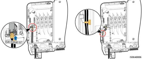
5. Tighten the thread-lock sealing nut and seal the waterproof connector.
